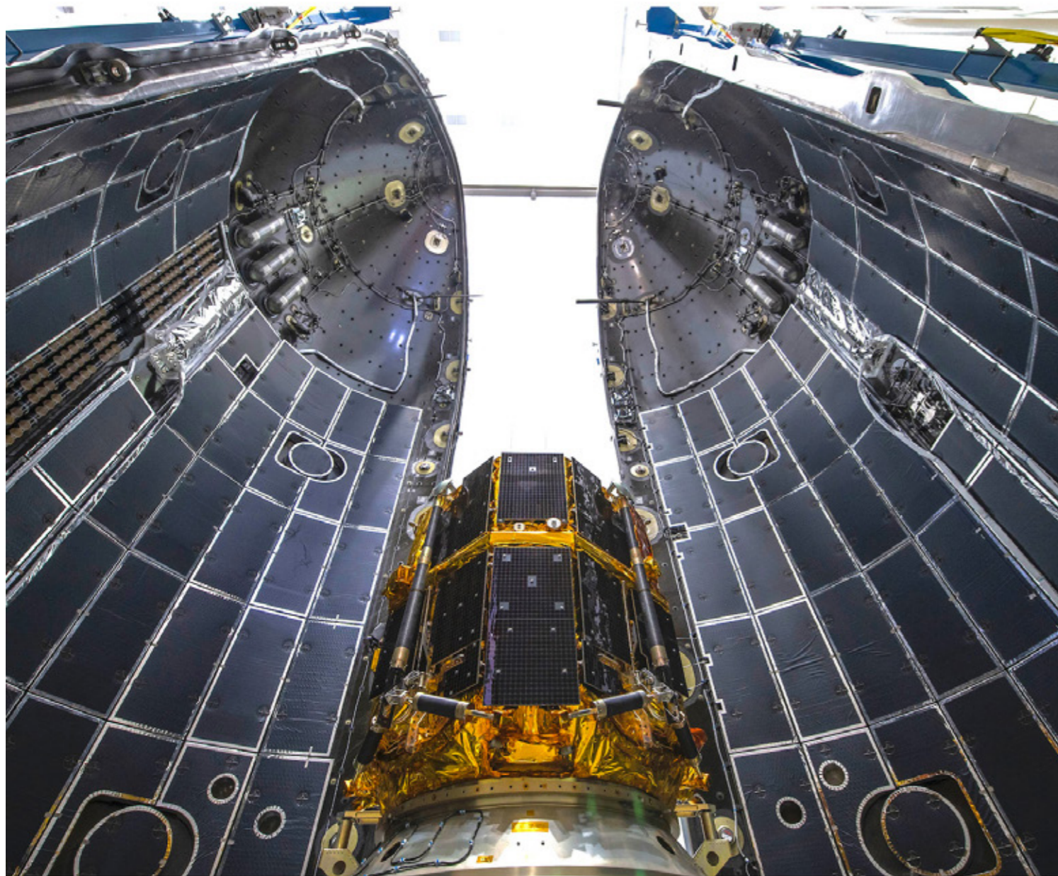
Series 1 Lander inside of launch vehicle fairing for Mission 1, late 2022.
